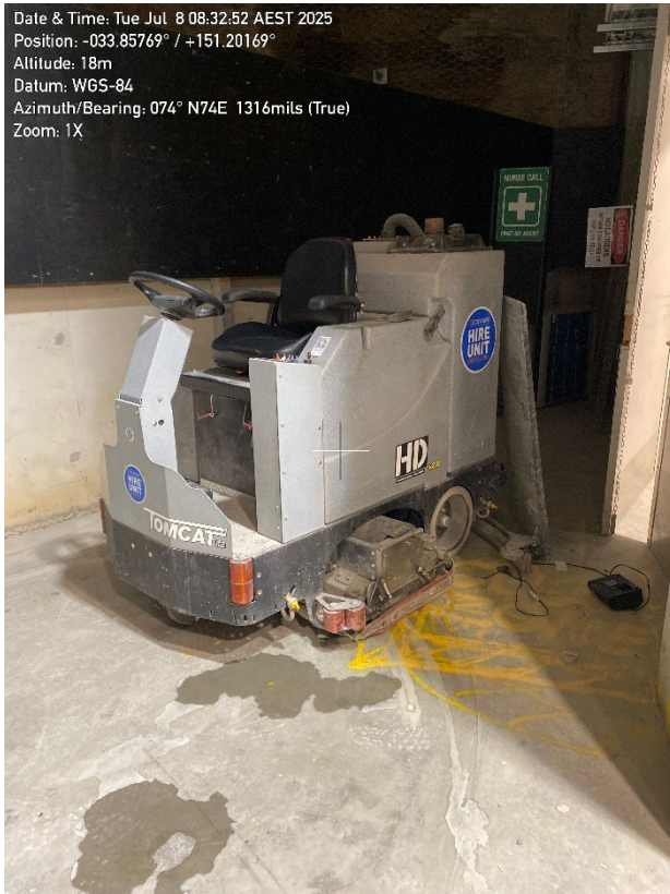
Photo 19 – Scrubber on the ground floor, which is used as required to remove dust.
