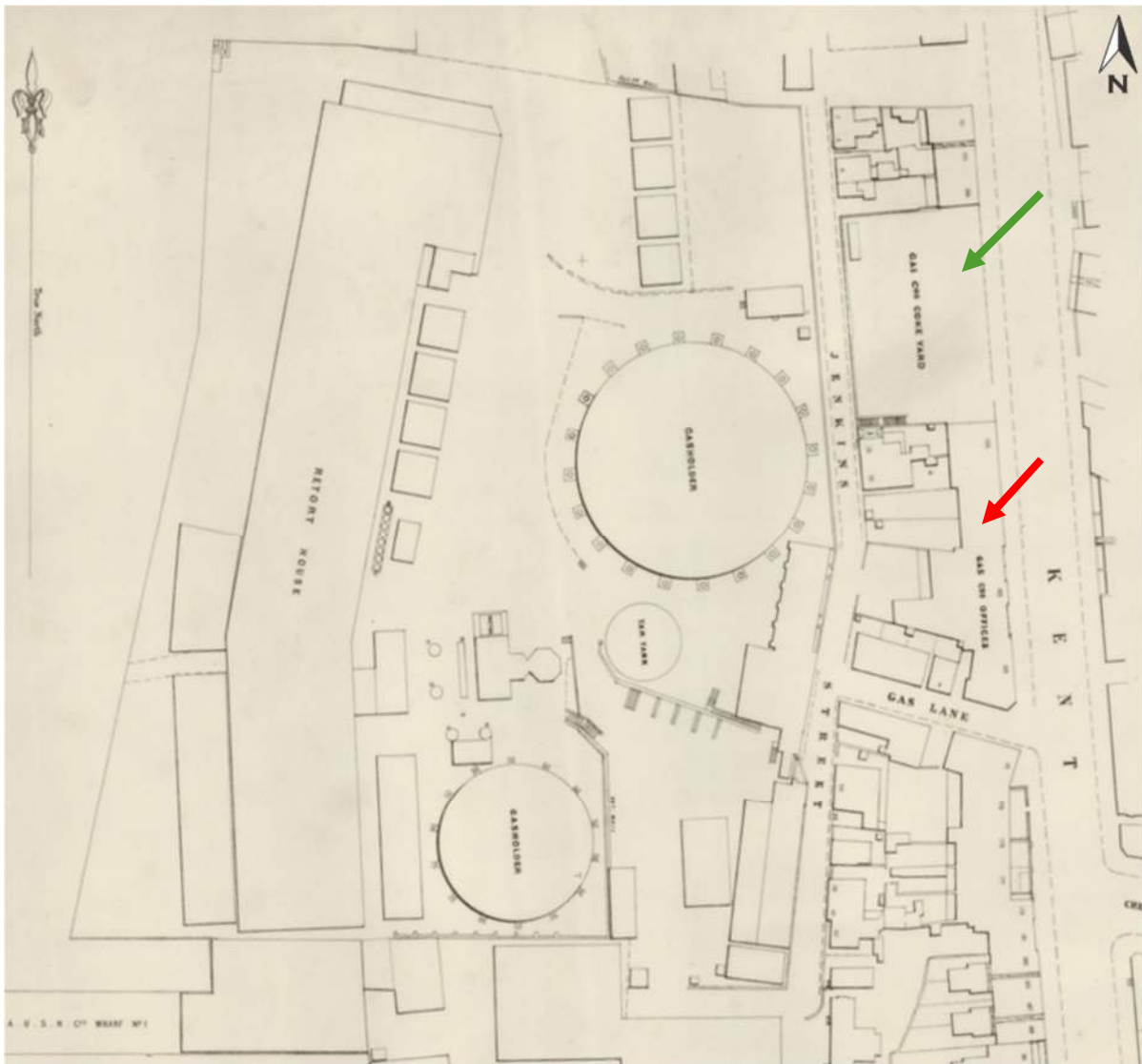
Figure 3.33: The AGL in 1891. Both the 1869-1870 and 1882 gasholders are shown, along with the tar tank, the new coke yard on Jenkins Street (green arrow) and the company offices on Kent Street (red arrow). SLNSW, Metropolitan Detail Series, Section 67. ML M Ser 4 811.17/1.
