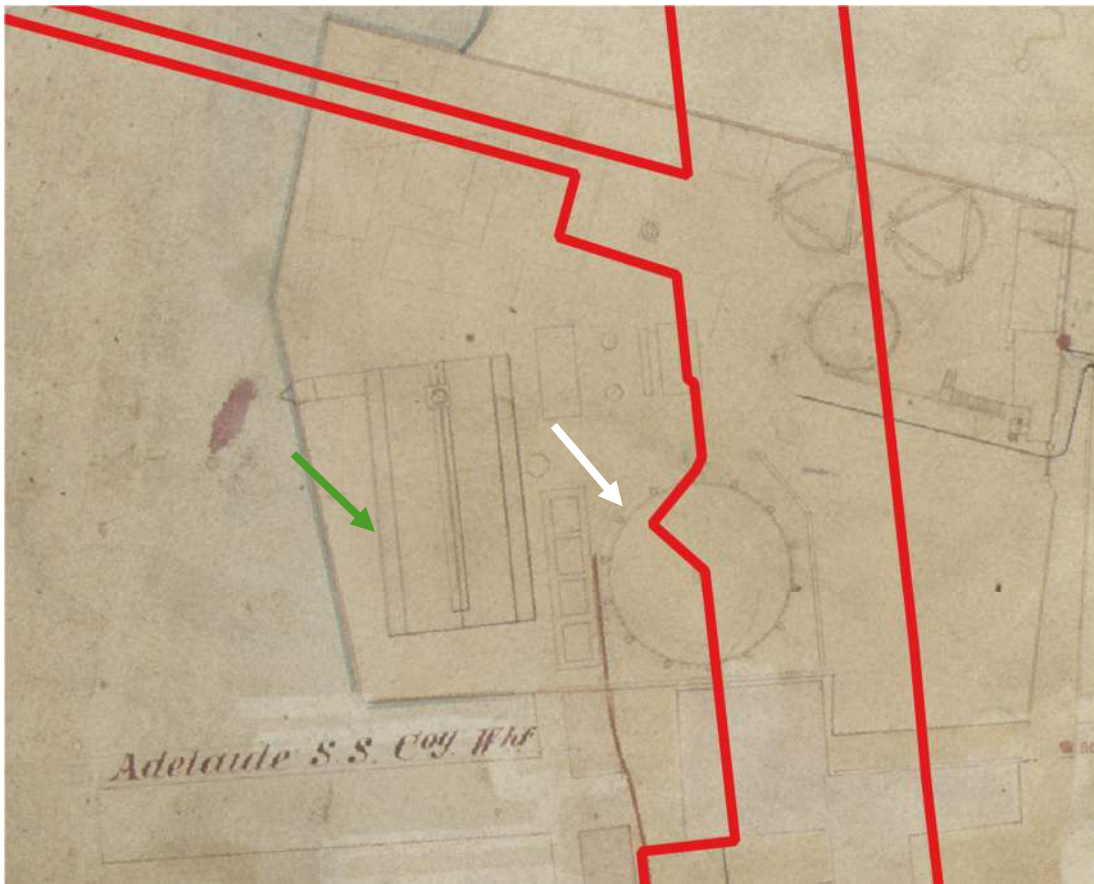
Figure 3.26: Detail of 1870 plan showing the new retort house (green arrow) to the south of the earlier retort complex (pencil outline), which was demolished during 1868. The 1870 gasholder (white arrow) co-exists with the three earlier gasholders, two of which are shown as disabled. 'Australian Gas Light Company Sydney plan of [gas] mains' Sheet 3. SLNSW ML, 811.17/1870/1.
